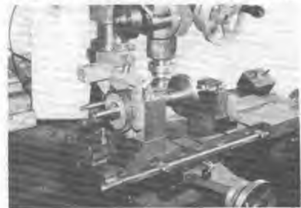
Fig. 66 Supporting the cutter arbor by an independent but matching tailstock.
